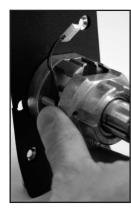
Rotate chassis 180 degrees, feed wire through rose plate, install rose plate 180 degrees from original orientation. Arrows on rose point toward latch.
