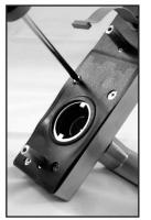
Remove lower back plate by removing (4) screws and remove lower thru bolt.
