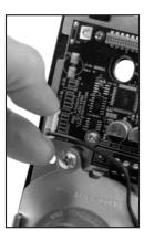
Disconnect motor wire, remove two rose plate screws and separate rose plate.
