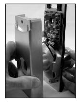
Re-install escutcheon plate and screws unless lock has external (hard wired) connections.
